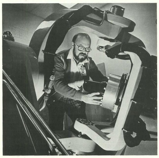
FLOYD FORSYTHE (1336) attaches a prototype guidance system module to the three-axis angular motion simulator in Sandia's Flight Simulation Laboratory. The simulator generates the angular rates of momentum expected in flight.
